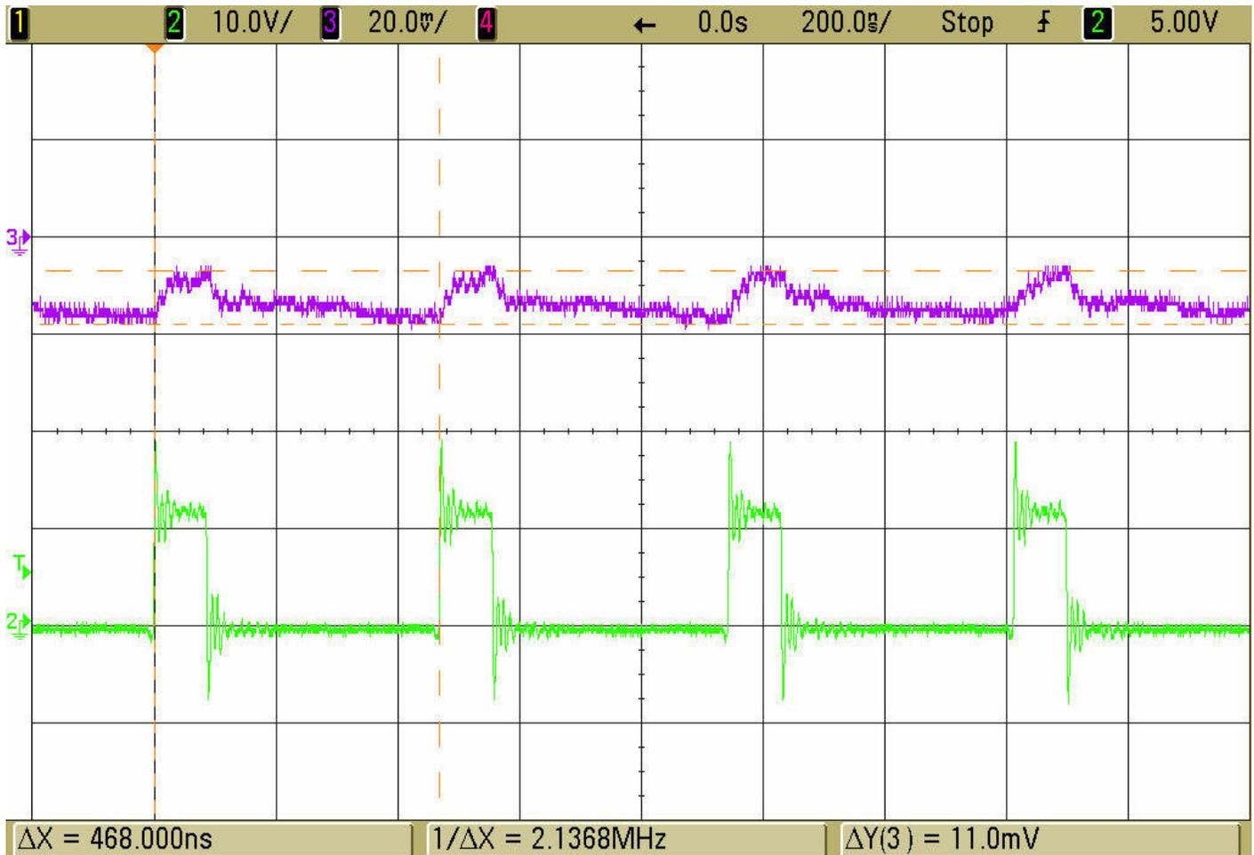
Figure 3. Switch Node & Output Ripple Voltage Waveforms
