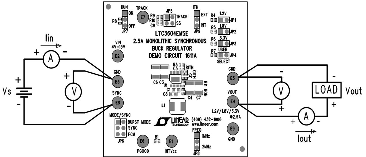
Figure 1. Proper Equipment Measurement Set-Up
