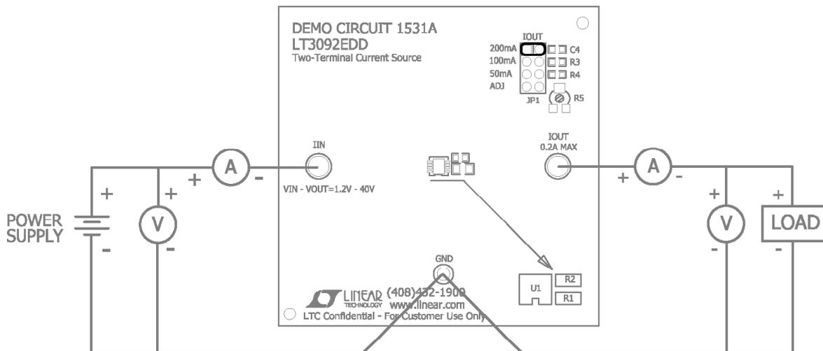
Figure 1. Proper Measurement Equipment Setup
