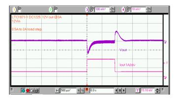
Figure 4. Fast transient response of DC1225 is achieved with a small ammount of output capacitance.
