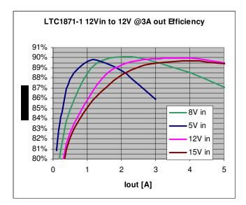
Figure 3. High efficiency of DC1225 allows the board to be used in thermally critical applications with outputs over 3A.
