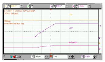
Figure 5. The DC1225 ramps the output slowly at startup without generating an input current surge.
