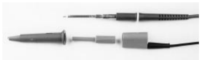
Figure 5. Scope Probe and Typical Measurement Setup
