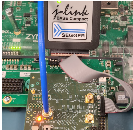
Figure 247. JLink Debugger with Adapter Connection
