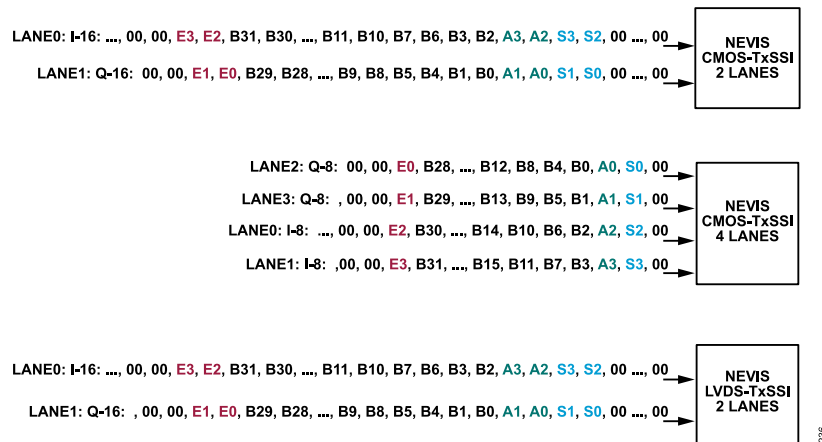
Figure 236. Tx-SSI Lane Mapping with Different Formats
