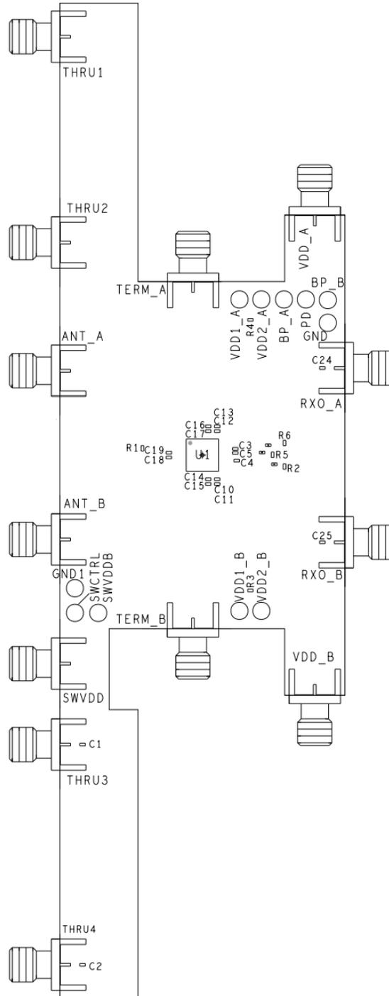
Figure 5. Evaluation Board Assembly Diagram
