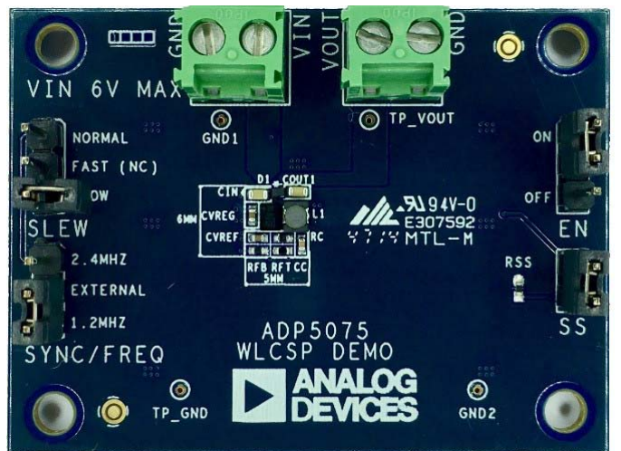
Figure 1. ADP5075CB-EVALZ Evaluation Board
