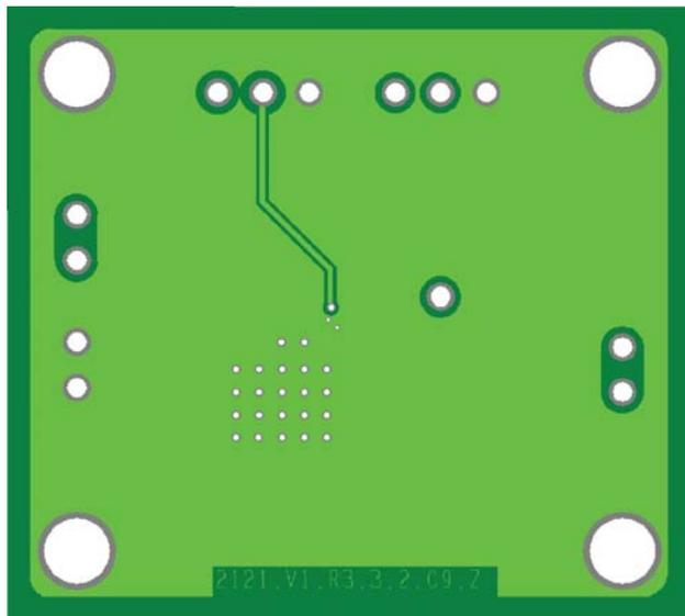
Figure 10. PCB Bottom Layer
