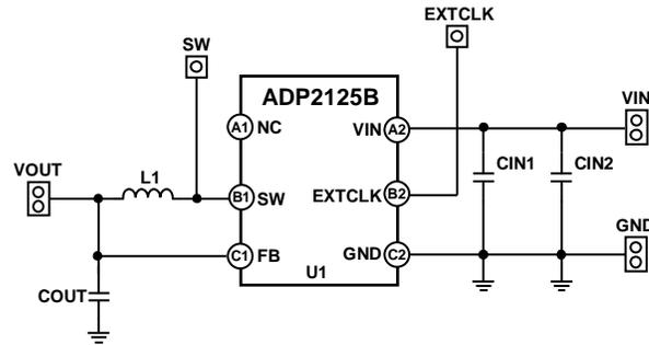
Figure 2. ADP2125 Evaluation Board Schematic
