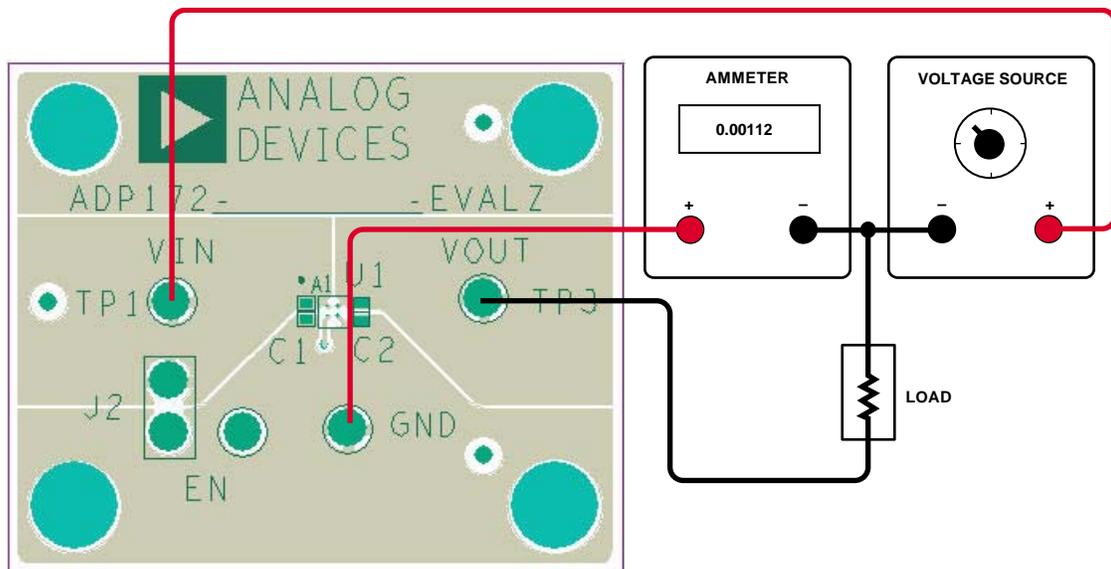
Figure 8. Ground Current Measurement Setup, WLCSP
