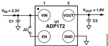
Figure 2. Evaluation Board Schematic, WLCSP
