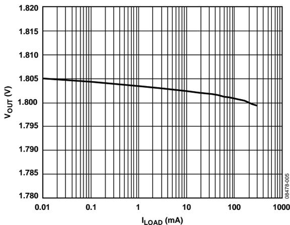
Figure 5. Output Voltage,  $V_{OUT}$  vs. Load Current,  $I_{LOAD}$  at  $V_{IN} = 2.3\text{ V}$ ,  $V_{OUT} = 1.8\text{ V}$ ,  $T_A = 25^\circ\text{C}$
