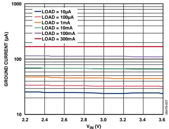
Figure 7. Ground Current vs. Input Voltage,  $V_{OUT} = 2.5\text{ V}$ ,  $T_A = 25^\circ\text{C}$
