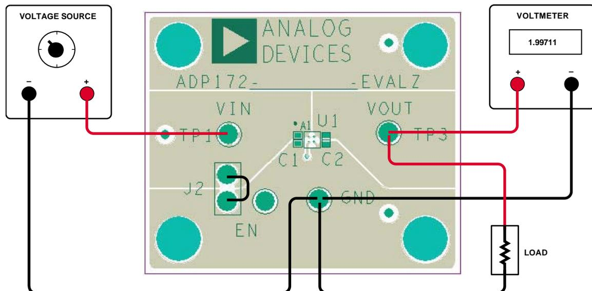
Figure 3. Output Voltage Measurement Setup, WLCSP
