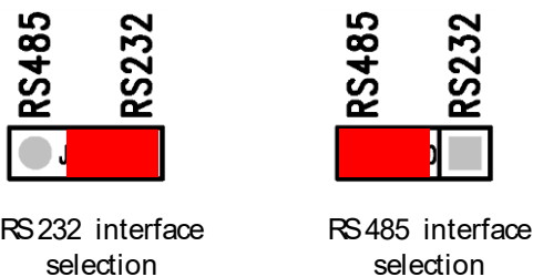
Figure 3.11 RS232/RS485 interface selection
