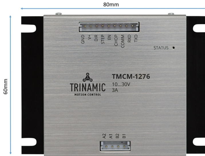
Figure 6: TMCM-1276 top view mechanical dimensions
