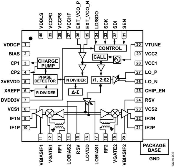
Figure 2. Simplified Block Diagram
