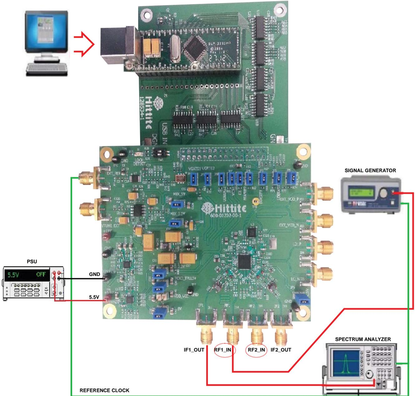
Figure 3. Test Setup for the HMC1190A Evaluation Board
