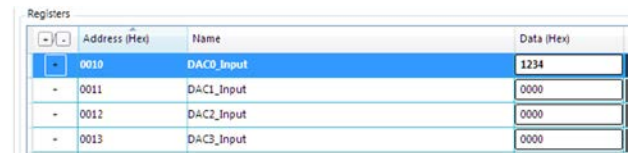
Figure 6. AD5679R Memory Map with Unapplied Changes in the DAC0_Input Register
