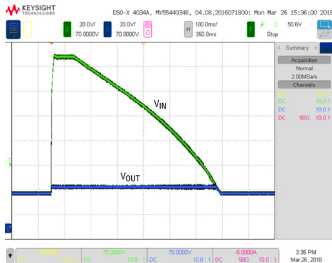
Figure 2. Output Response Waveform with 28V to 140V Input Surge (CH2 V_{IN} 20V/DIV, CH3 V_{OUT} 20V/DIV, 100ms/DIV)
