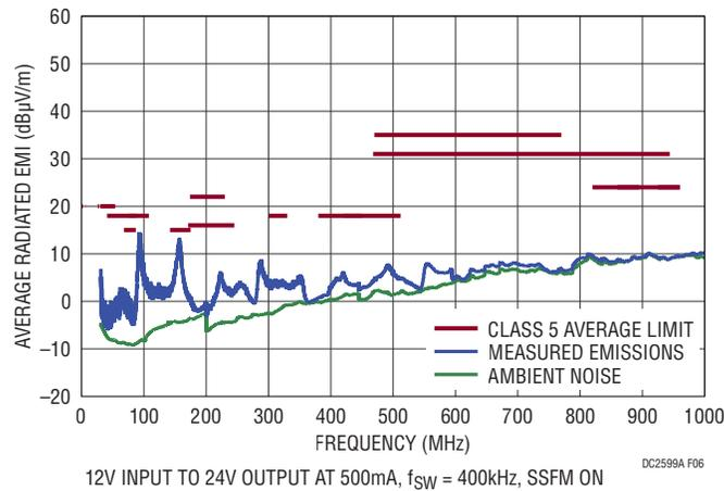
**Figure 6. CISPR25 Radiated Emissions Test, Average Detection**
