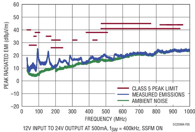
**Figure 5. CISPR25 Radiated Emissions Test, Peak Detection**
