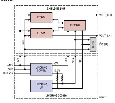
Figure 11. DC2467 Block Diagram
