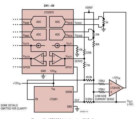
Figure 13. LTC2970 Interface to -5V Rail
