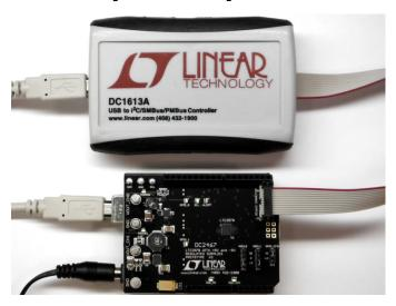
Figure 7. DC2467 with DC1613 Dongle Attached
