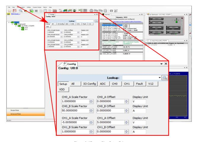
Figure 9. LTpowerPlay Setup Tab
