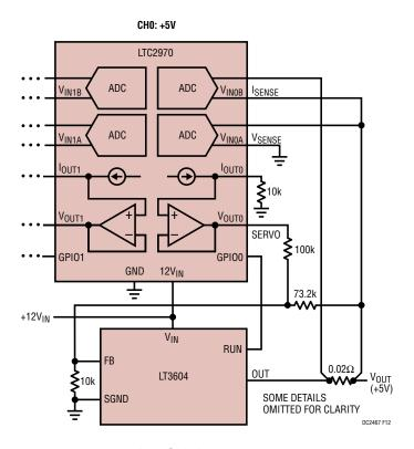
Figure 12. LTC2970 Interface to +5V Rail
