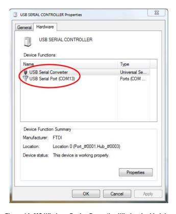
Figure 14. MS Windows Device Properties Window for Linduino
