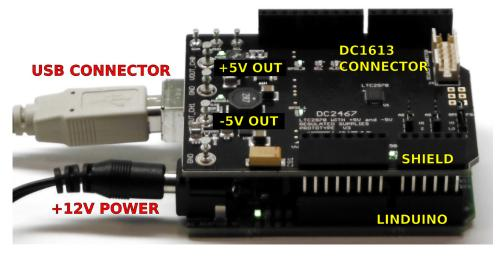
Figure 1. DC2467 Shield Mounted on the DC2026 Linduino
