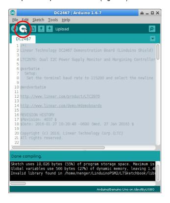
Figure 3. Press the Compile and Upload Button
