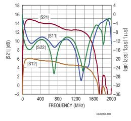
Figure 2. Demo Board S-Parameters
