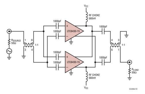
Figure 1. DC2090A Two LTC6430-15s in Parallel Simplified Schematic
