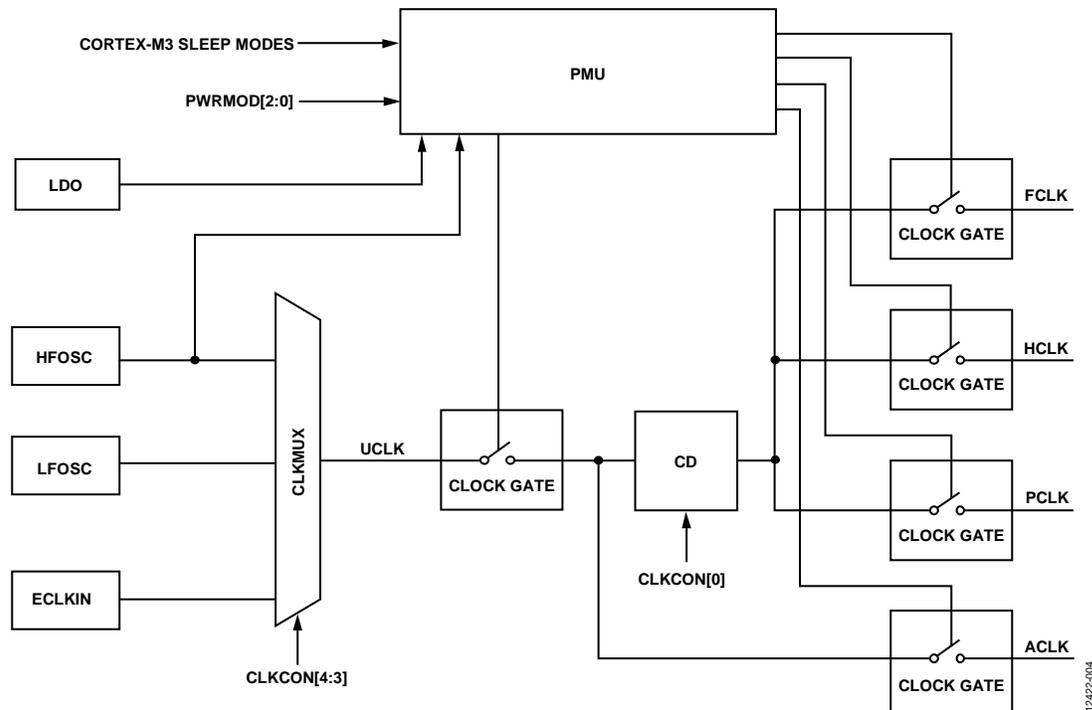
Figure 3. System Clock Architecture Block Diagram
