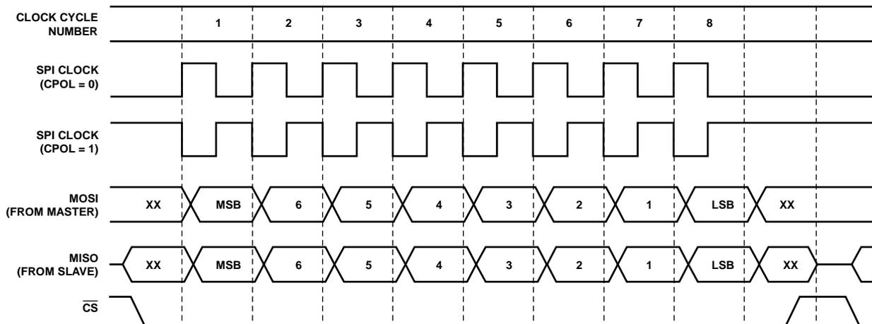
Figure 29. SPI Transfer Protocol, CPHA = 1
