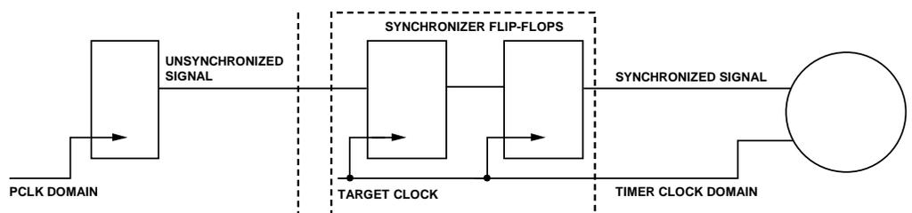
Figure 23. Synchronizer for Signals Crossing Clock Domains
