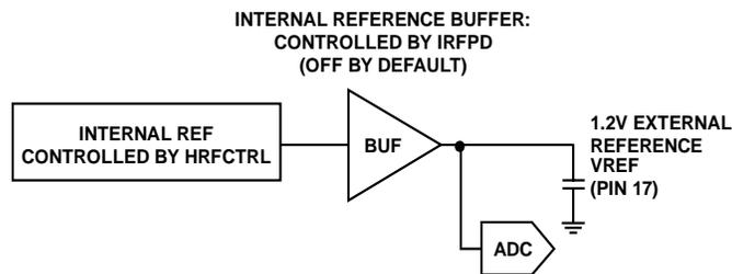
Figure 18. ADC Reference Configuration
