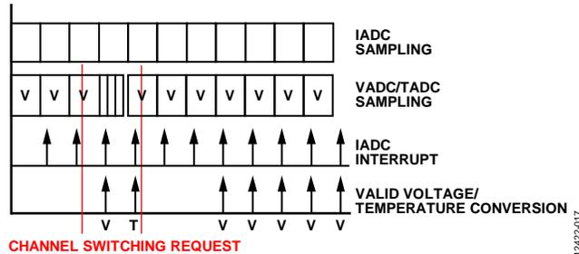
Figure 17. Fast Temperature Mode, Chop Off (ADCFLT = 0x07)
