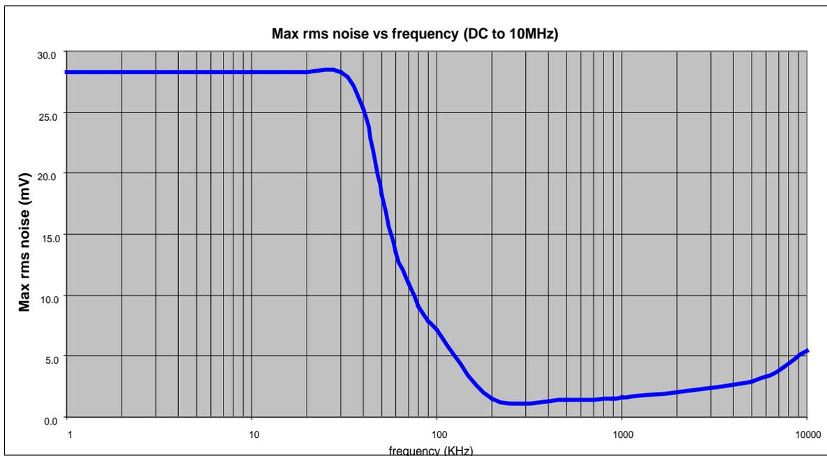
Figure 23 LC Filter Transfer Curve
