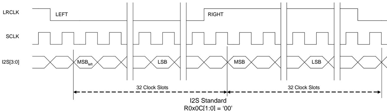
Figure 11 I2S Standard Audio – 16-bit samples only
