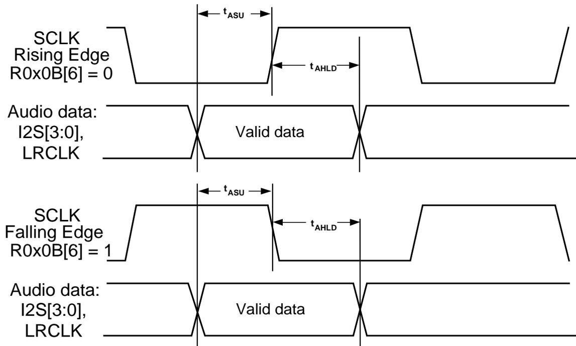
Figure 4 Timing for S/PDIF Audio Interface
