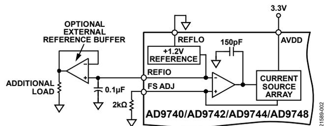
Figure 3. Internal Reference Configuration
