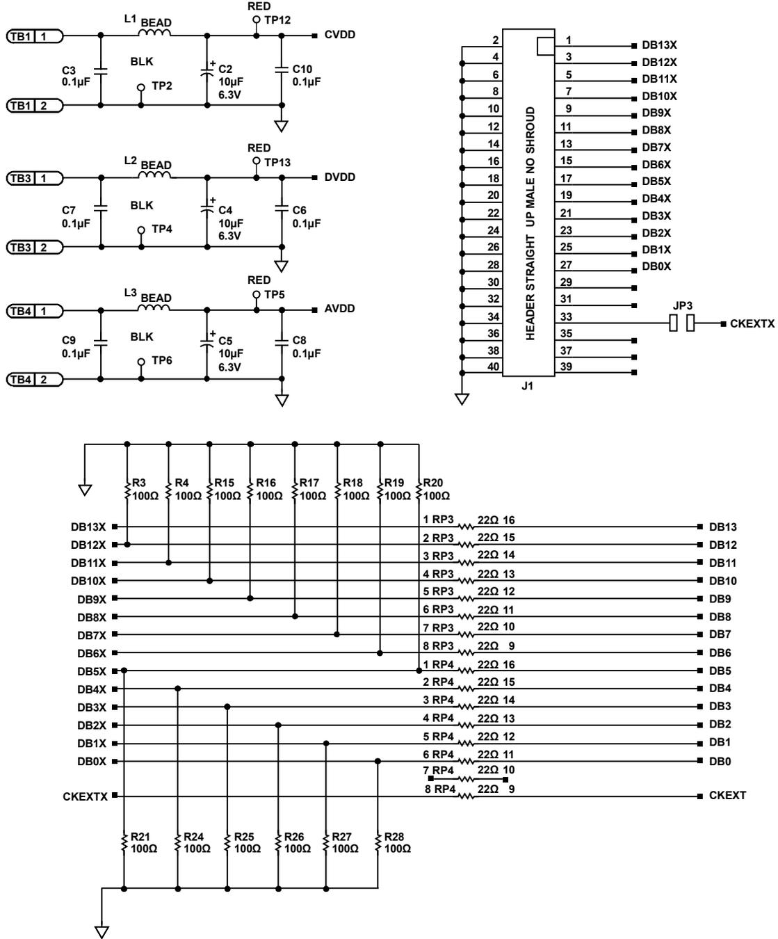
Figure 32. AD9740ACP-PCBZ/AD9742ACP-PCBZ/AD9744ACP-PCBZ/AD9748ACP-PCBZ LFCSP Evaluation Board Schematic—Power Supply and Digital Inputs
