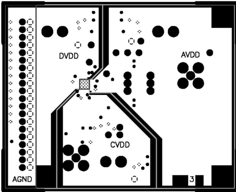
Figure 38. AD9740ACP-PCBZ/AD9742ACP-PCBZ/AD9744ACP-PCBZ/AD9748ACP-PCBZ LFCSP Evaluation Board Layout—Power Plane
