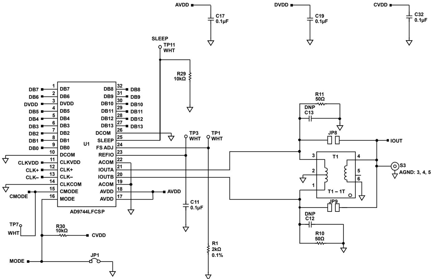
Figure 33. AD9740ACP-PCBZ/AD9742ACP-PCBZ/AD9744ACP-PCBZ/AD9748ACP-PCBZ LFCSP Evaluation Board Schematic—Output Signal Conditioning
