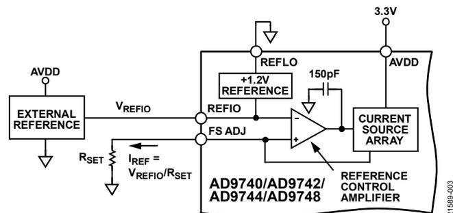
Figure 4. External Reference Configuration
