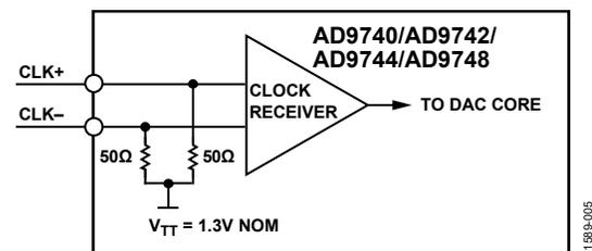
Figure 6. Clock Termination in PECL Mode
