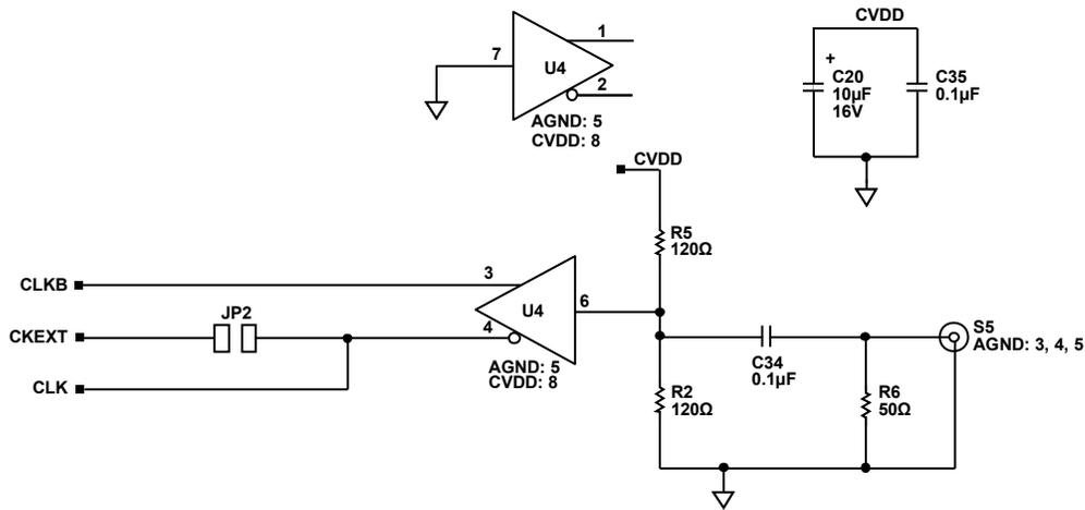
Figure 34. AD9740ACP-PCBZ/AD9742ACP-PCBZ/AD9744ACP-PCBZ/AD9748ACP-PCBZ LFCSP Evaluation Board Schematic—Clock Input
