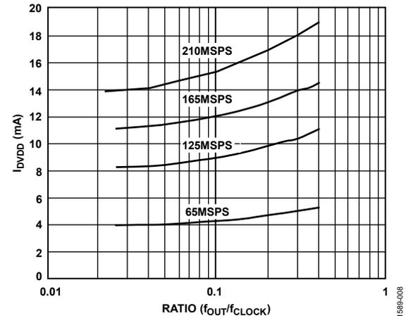
Figure 9.  $I_{DVDD}$  vs. Ratio ( $f_{OUT}/f_{CLOCK}$ ) at  $DVDD = 3.3 V$
