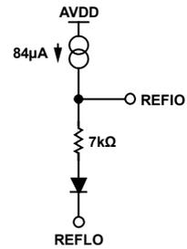
Figure 2. Equivalent Circuit of Internal Band Gap Reference
