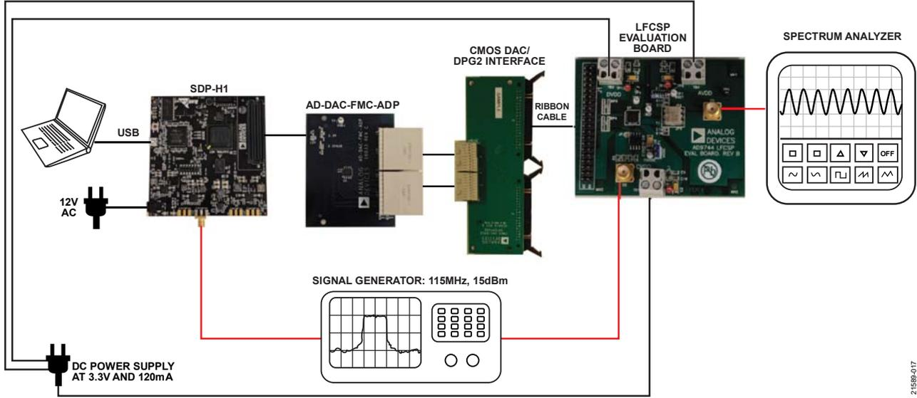
Figure 18. Hardware Connections
