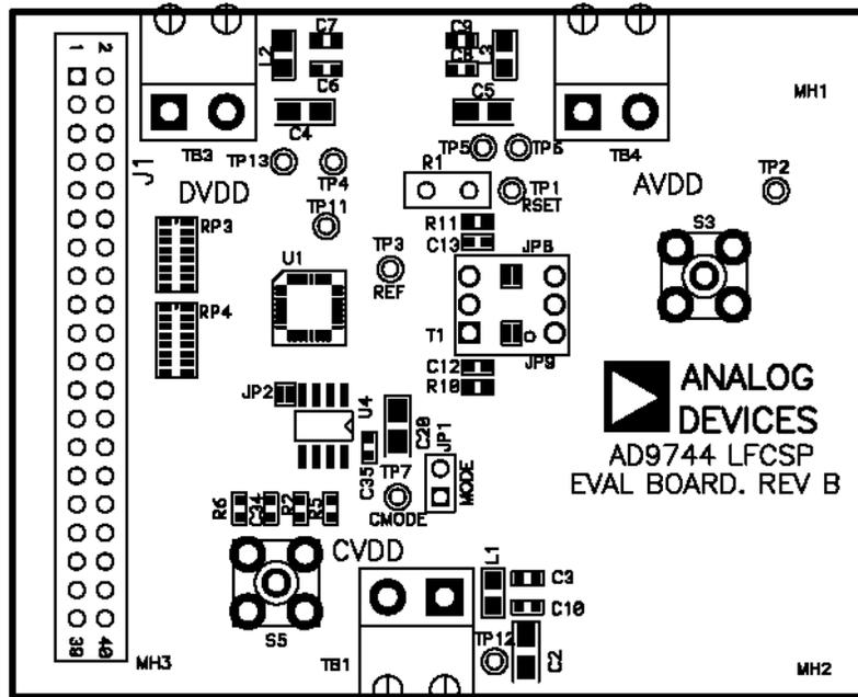
Figure 39. AD9740ACP-PCBZ/AD9742ACP-PCBZ/AD9744ACP-PCBZ/AD9748ACP-PCBZ LFCSP Evaluation Board Layout Assembly—Primary Side
