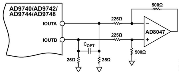
Figure 12. DC Differential Coupling Using an Op Amp
