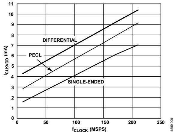
Figure 10.  $I_{CLKVDD}$  vs.  $f_{CLOCK}$  and Clock Mode
