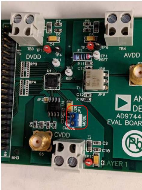
Figure 19. Evaluation Board JP1 Jumper Shunt
