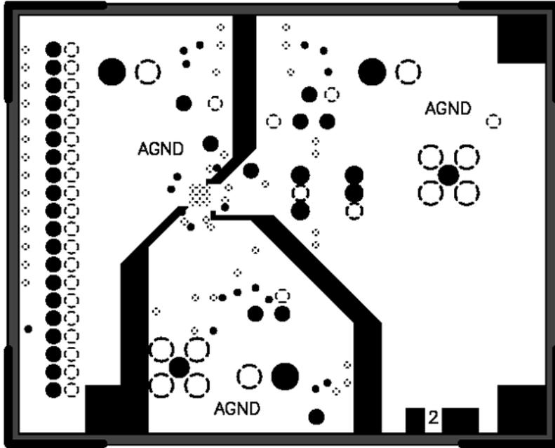
Figure 37. AD9740ACP-PCBZ/AD9742ACP-PCBZ/AD9744ACP-PCBZ/AD9748ACP-PCBZ LFCSP Evaluation Board Layout—Ground Plane
