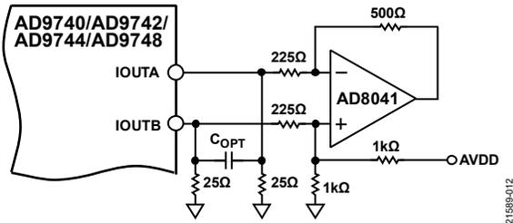
Figure 13. Single-Supply DC Differential Coupled Circuit
