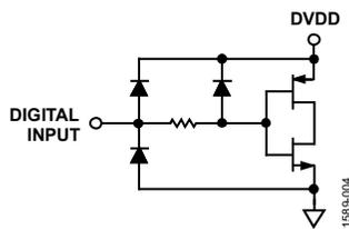
Figure 5. Equivalent Digital Mode
