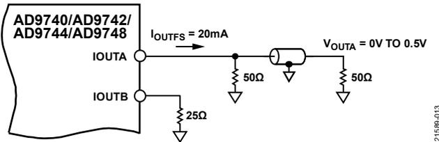
Figure 14. 0 V to 0.5 V Unbuffered Voltage Output
