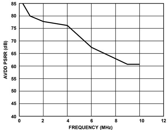
Figure 16. AVDD PSRR vs. Frequency
