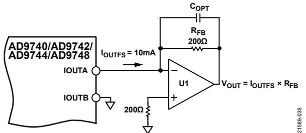
Figure 15. Unipolar Buffered Voltage Output
