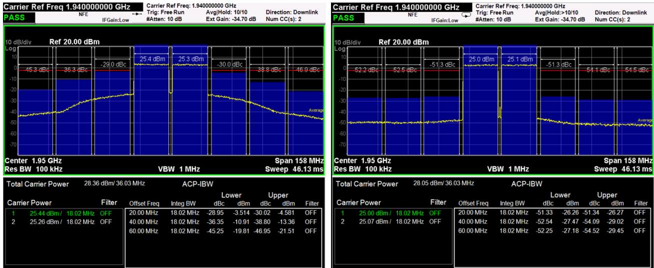
Figure 2. SKY66399-11 @ 1950 MHz, 20 MHz ETM3.1 signal 2Carrier before/after DPD
