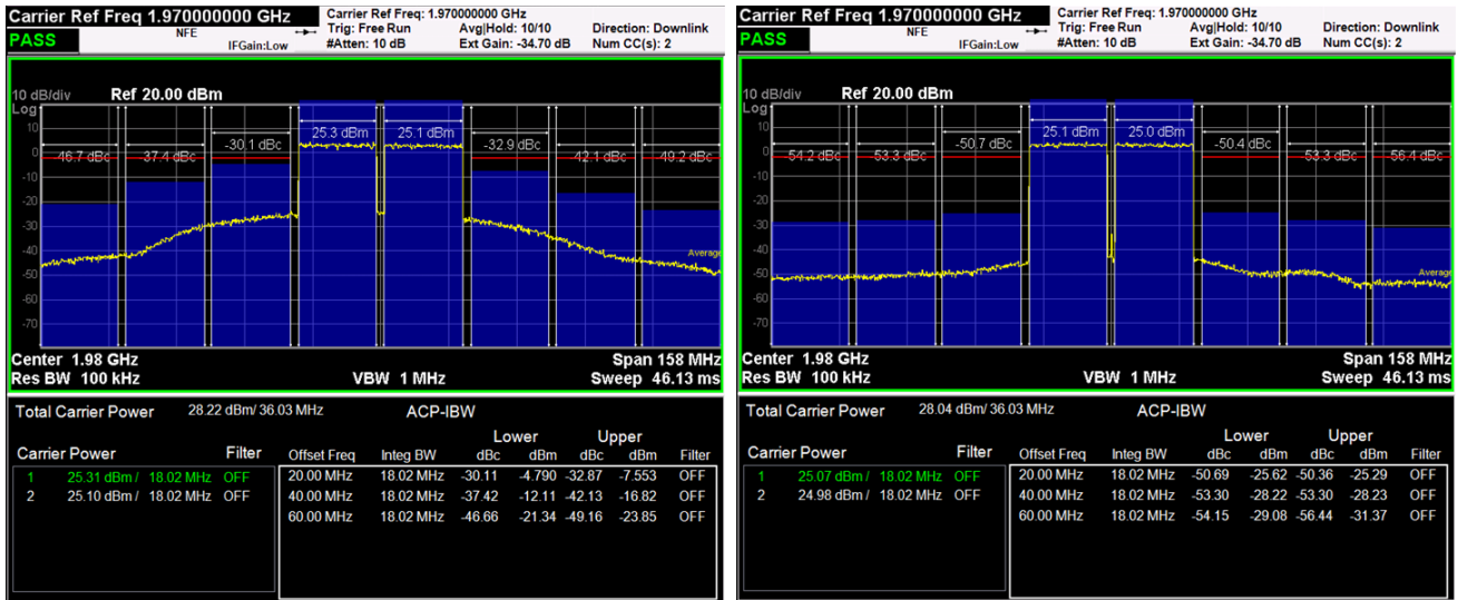
Figure 3. SKY66399-11 @ 1980 MHz, 20 MHz ETM3.1 signal 2Carrier before/after DPD
