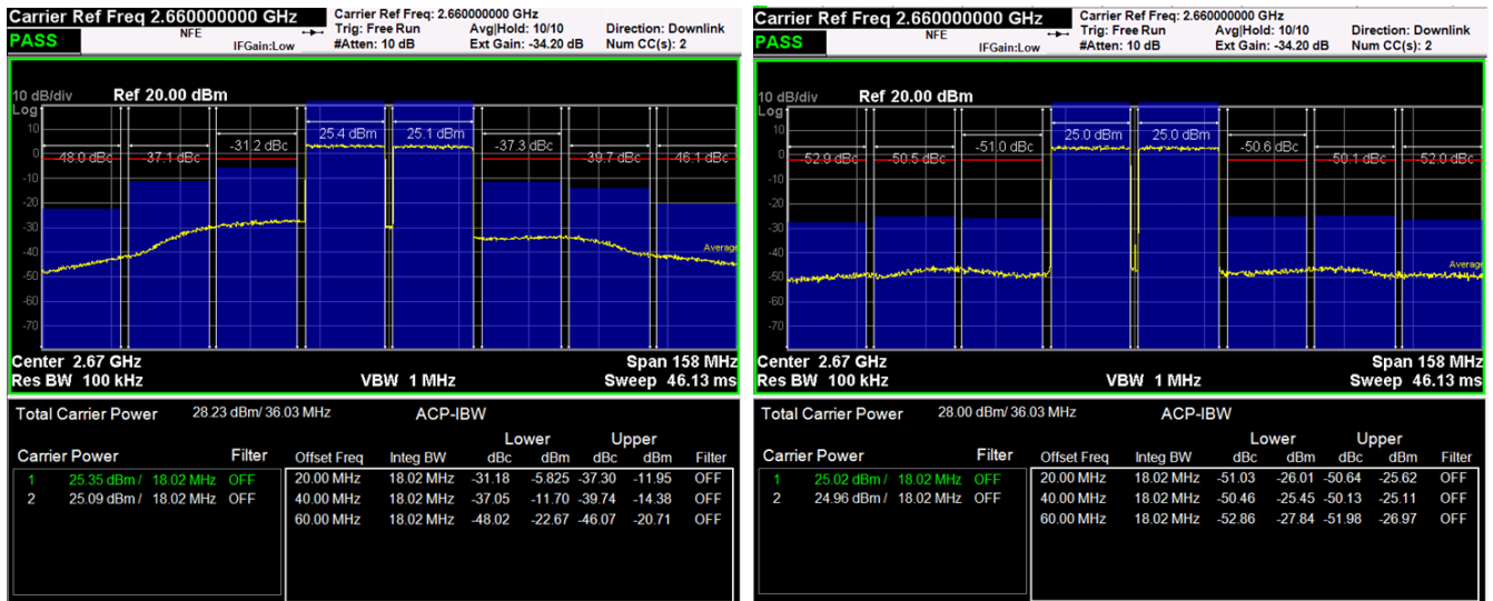
Figure 3. SKY66397-11 @ 2670 MHz, 20 MHz ETM3.1 signal 2Carrier before/after DPD
