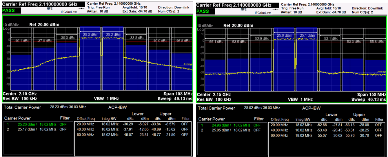
Figure 3. SKY66394-11 @ 2150 MHz, 20 MHz ETM3.1 signal 2Carrier before/after DPD
