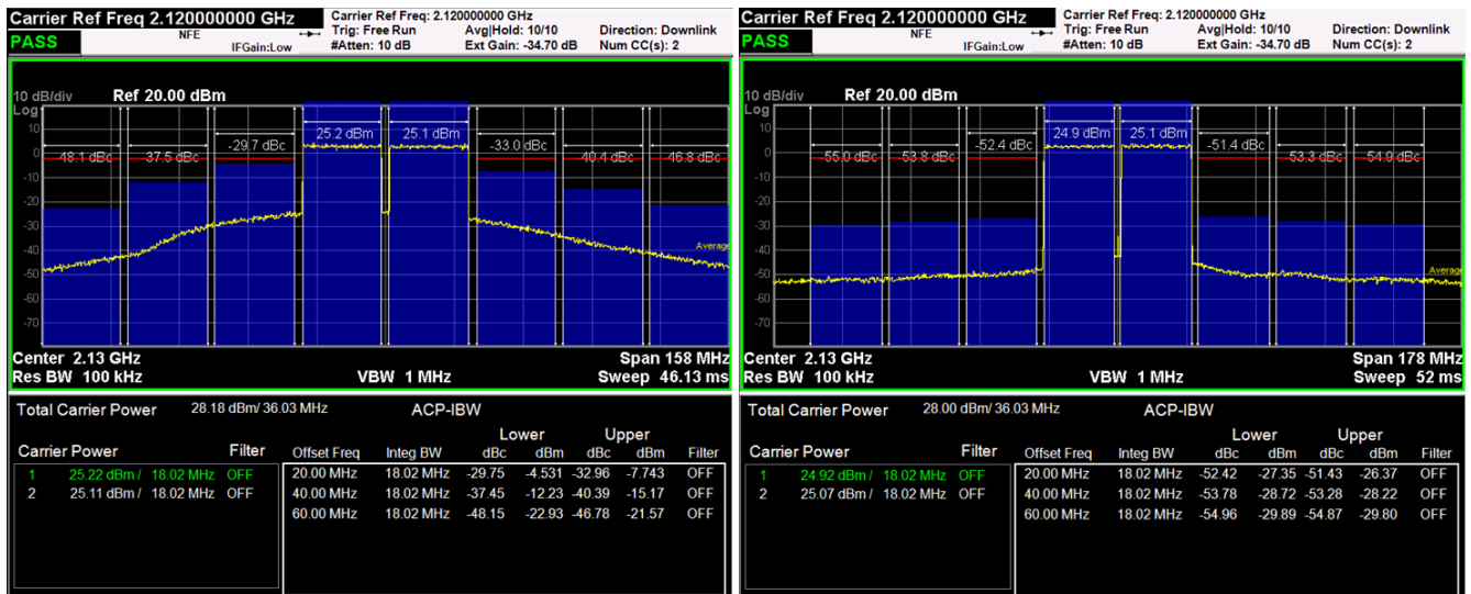
Figure 1. SKY66394-11 @ 2130 MHz, 20 MHz ETM3.1 signal 2Carrier before/after DPD
