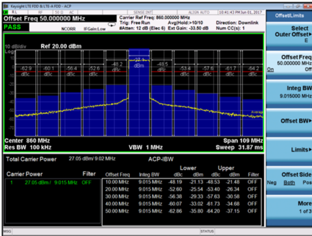
Figure 4: Wideband Spectrum Analyser Plot: Frequency 860 MHz, 10MHz ETM3.1 Signal
