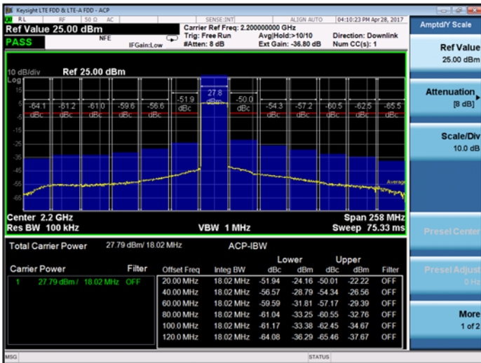
Figure 5: Wideband Spectrum Analyser Plot: Frequency 2200MHZ, 20MHz ETM3.1 Signal
