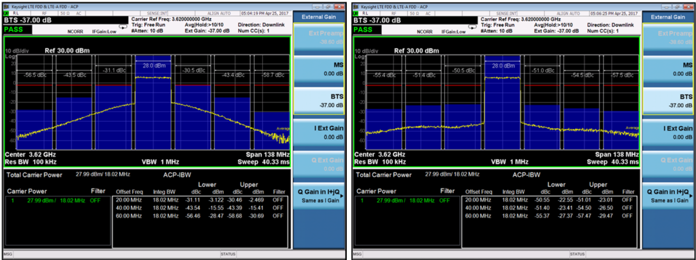
Figure 2. Frequency 3620MHz, 20MHz ETM3.1 Signal
