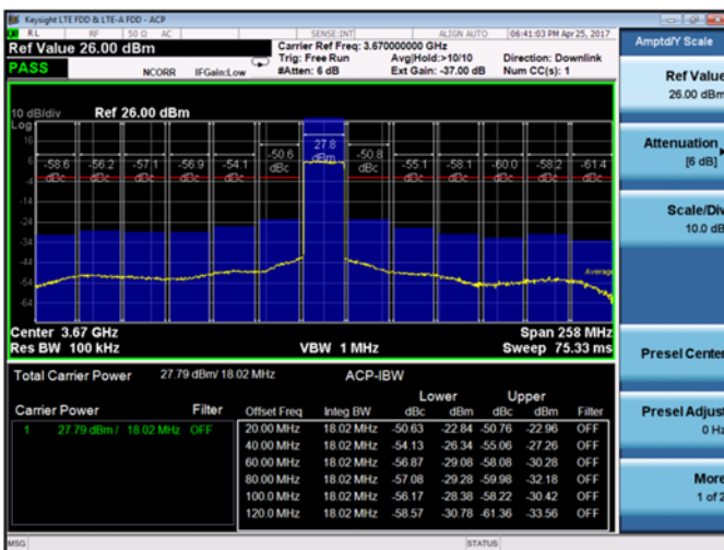
Figure 6. Wideband Spectrum Analyser Plot: Frequency 3670MHZ, 20MHz ETM3.1 Signal
