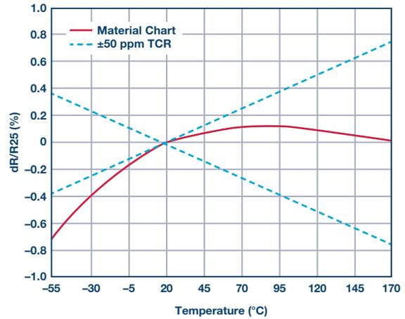
Figure 2. Parabolic TCR curve of Bourns model CSS4J-4026R current sense resistor.
