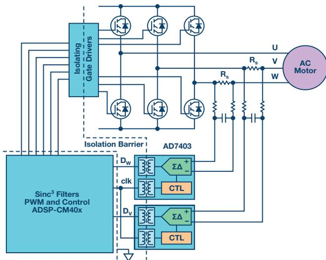
Figure 1. Block diagram of three phase motor drive with digital isolation and sense resistors.
