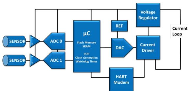
Figure 1. Smart Transmitter Signal Chain
