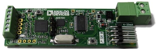
Figure 4. HART Registered Field Instrument Demo Board
