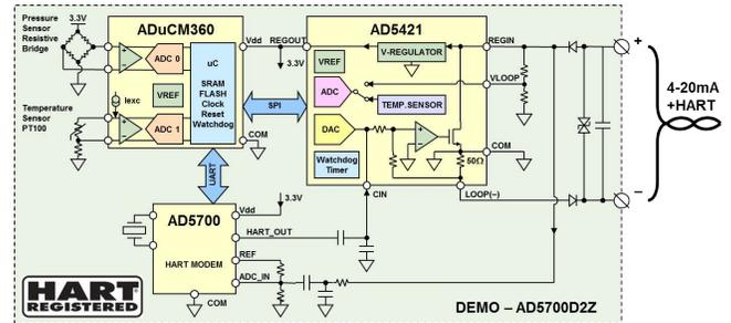
Figure 2. HART Enabled Field Instrument Demo Block Diagram
