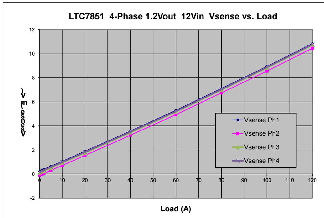
**Figure 3. Four Phase Current Balance for a Single 1.2V/120A Output**
