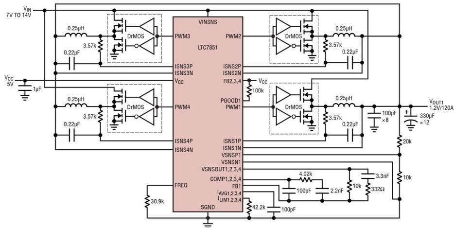
Figure 1. LTC7851 Simplified Schematic Delivering a Single 1.2V/120A Output
