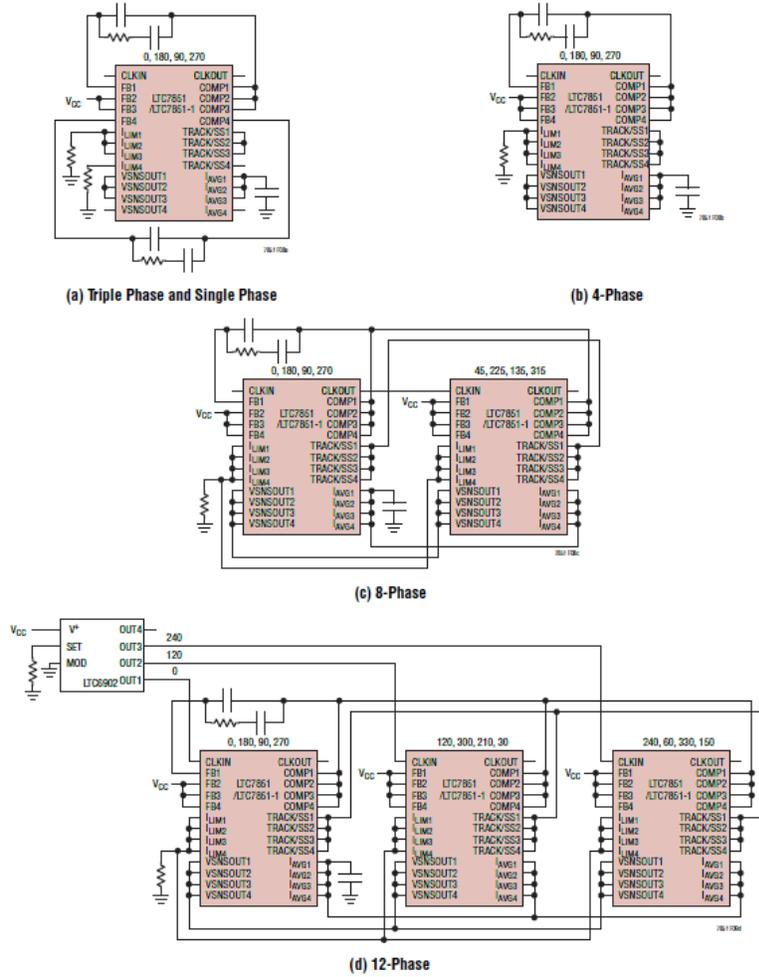
Figure 4. LTC7851 Multiple Phase Configurations
