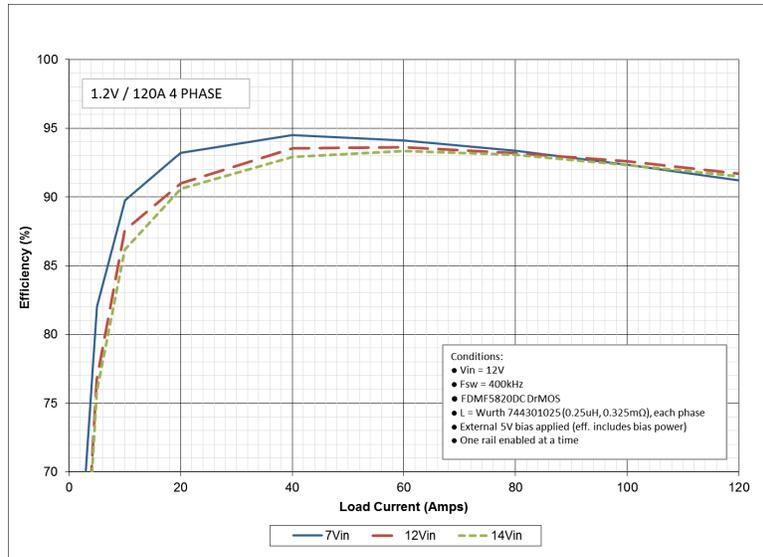
**Figure 2. LTC7851 Efficiency Curves for a 7V, 12V & 14V Input to a Single 1.2V/120A Output**
