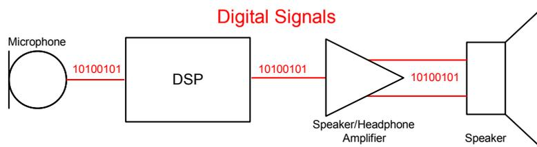
Figure 2. Fully Digital Audio Signal Chain
