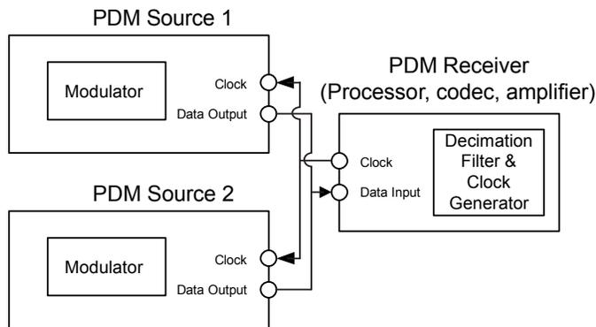
Figure 4. Dual-Source PDM Connection Diagram
