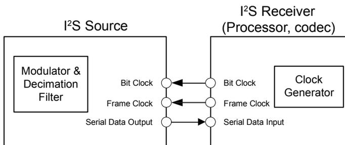
Figure 3. I<sup>2</sup>S Connection Diagram, Receiver as Master
