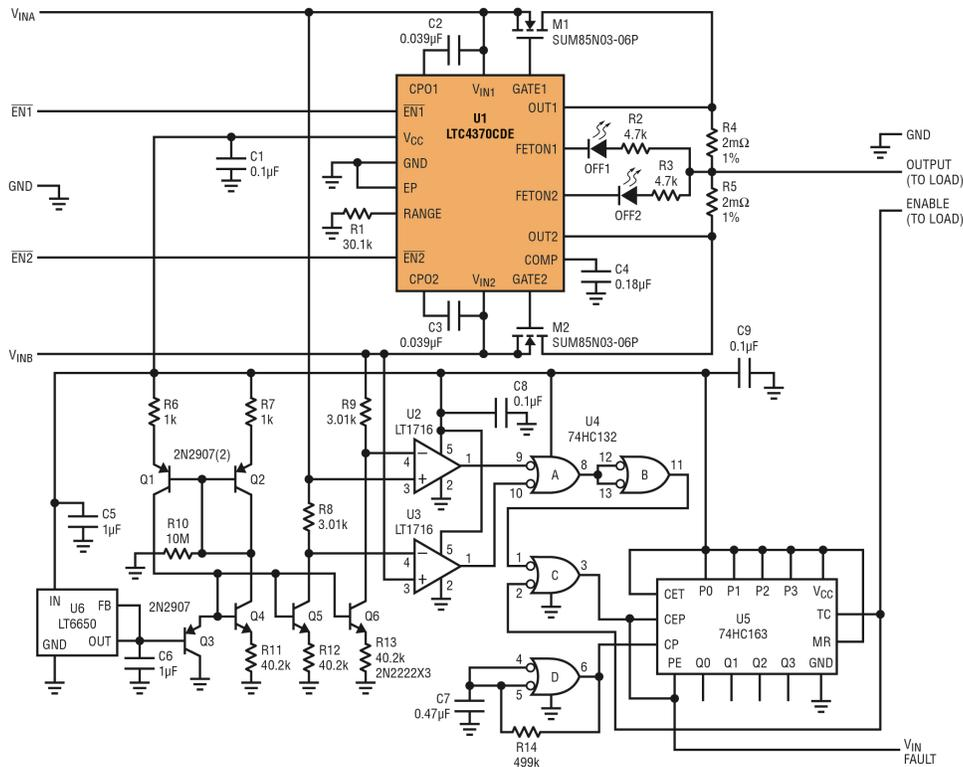
Figure 2. Complete load sharing design
