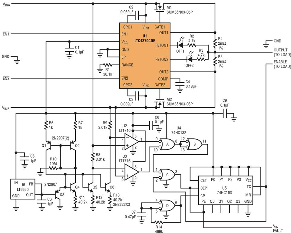
Figure 2. Complete load sharing design
