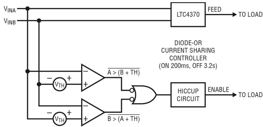
Figure 1. Block diagram of current summing circuitry
