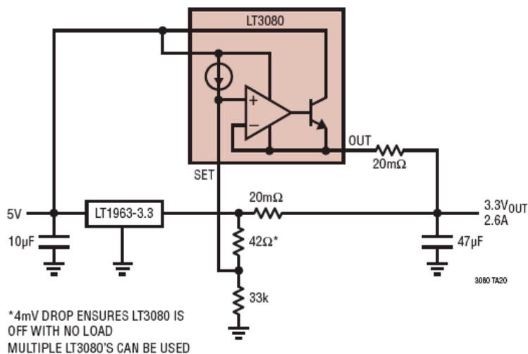
Figure 3. Boosting the output current of a fixed regulator
