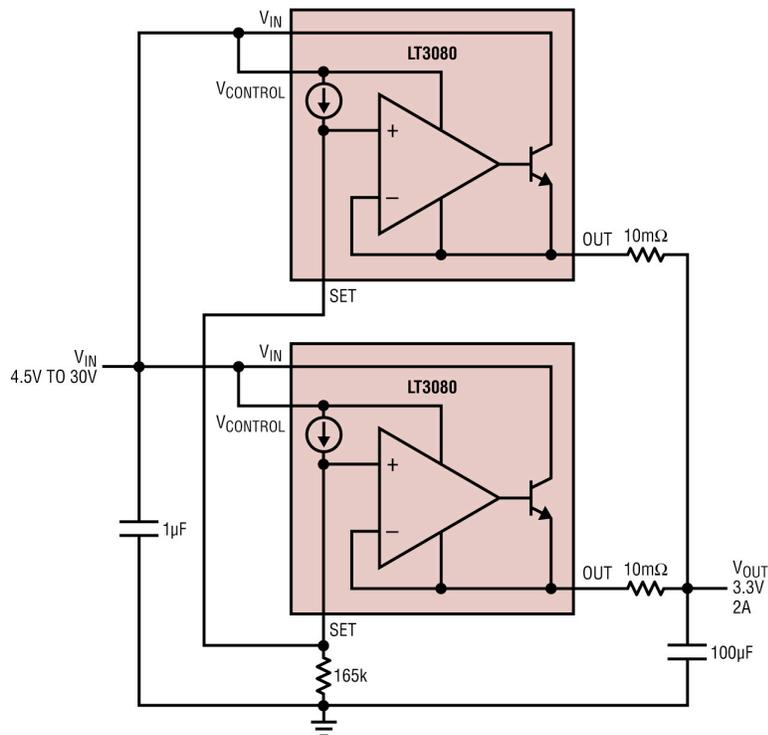
Figure 2 Parallel operation of the LT3080
