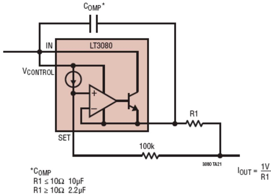
Figure 4 shows 2 “two terminal” current source configurations for the LT3080.
