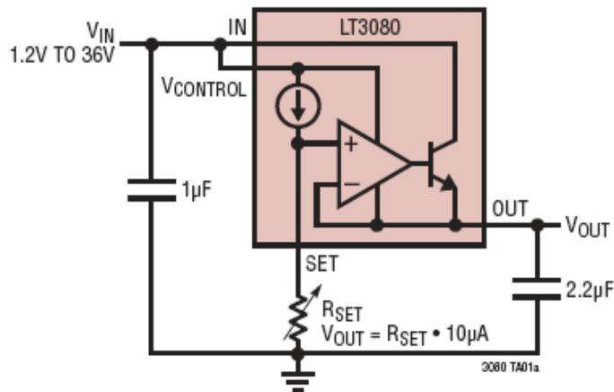
Fig. 1 Basic operation of the LT3080
