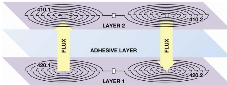
Figure 5. isoPower Transformer Configuration
