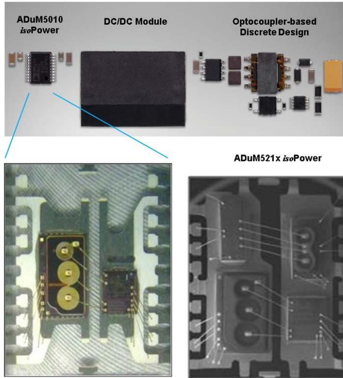
Figures 1. (a) Size Comparison of Various Isolated Power Implementations; (b) Inside Look of ADuM5010, a 150 mW Fully Integrated Dc-to-Dc Converter; (c) Inside Look of ADuM521x, a Dual Channel Isolated with Integrated Dc-to-Dc Converter
