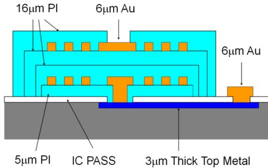
Figure 3. Cross Section of *isoPower* Transformers
