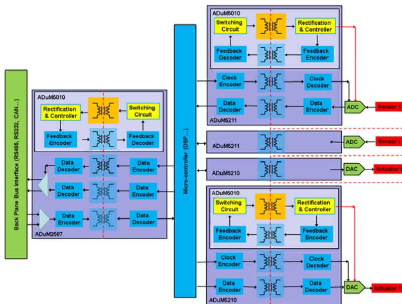
Figure 6. Fully Isolated Industrial Measurement and Control System Using *isoPower*
