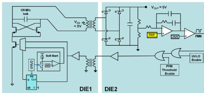
Figure 2. Schematic for Isolated Power Transfer Using Microtransformers
