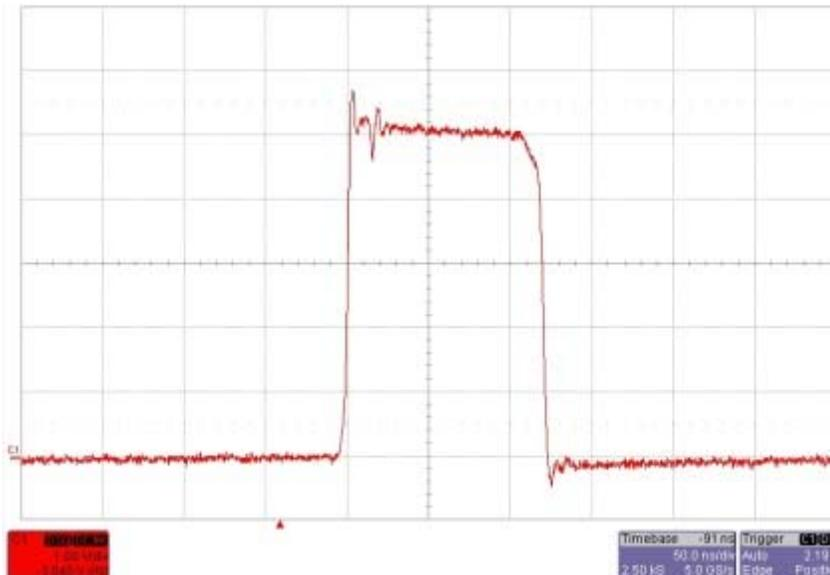
**Figure 3: Buck regulator switching @2MHz, reduced speed rise & fall times**
