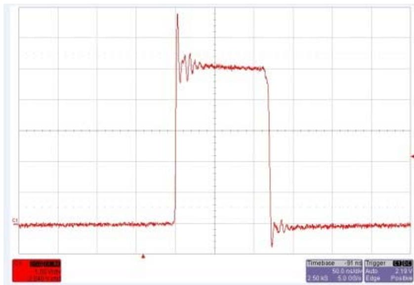
**Figure 2: Buck regulator switching @2MHz with full speed rise & fall times**
