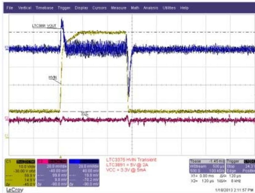
**Figure 5: LTC3375 high voltage transient performance**
