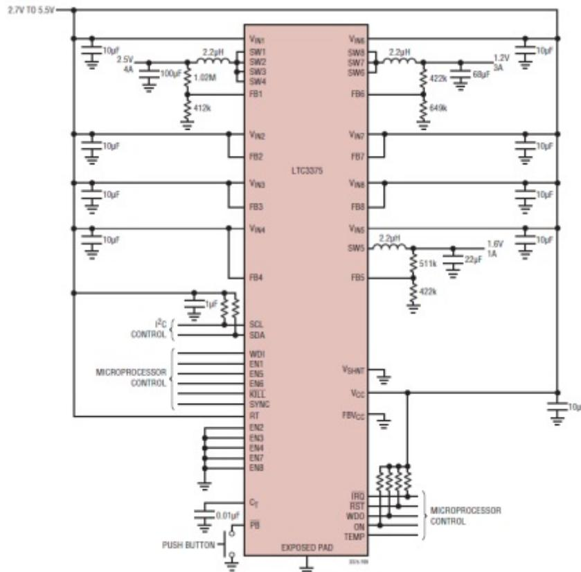
**Figure 1: LTC3375 simplified 3-output 4A / 3A / 1A block diagram**
