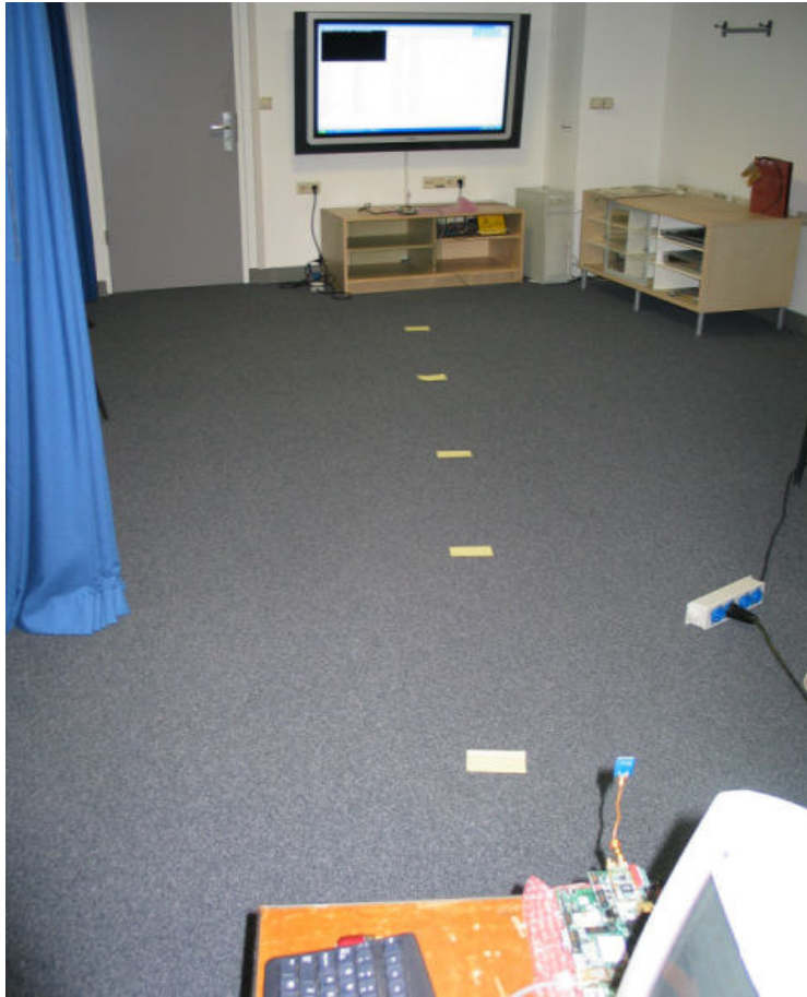
Figure 7 PULSERS VHDR: TX (bottom in the picture) and RX (top) components 6 meters apart.
