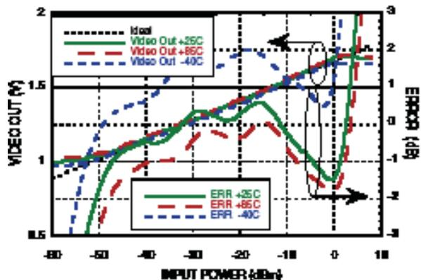
Figure 5. This plot shows the video output and log error vs. input power at 20 GHz for the HMC613LC4B SDLVA.
