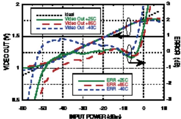
Figure 4. This plot shows the video output and log error vs. input power at 2 GHz for the HMC613LC4B SDLVA.
