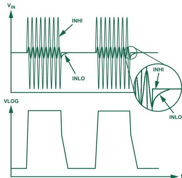
Figure 6. A closer look at signals at INHI and INLO when using circuit shown in Figure 4b.
