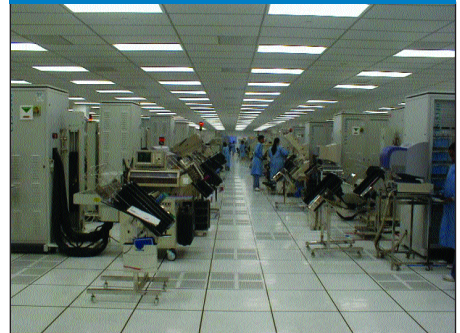
Fig 4: Automatic test equipment for production of ICs
