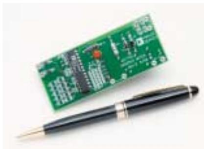
Actual size of a single IC kWh measurement base unit.
