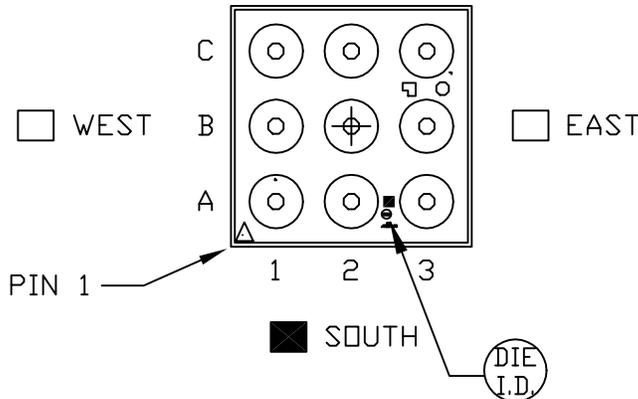
SELECT THE BOX INDICATING THE WAFER FLAT SIDE WITH RESPECT TO PIN 1.
