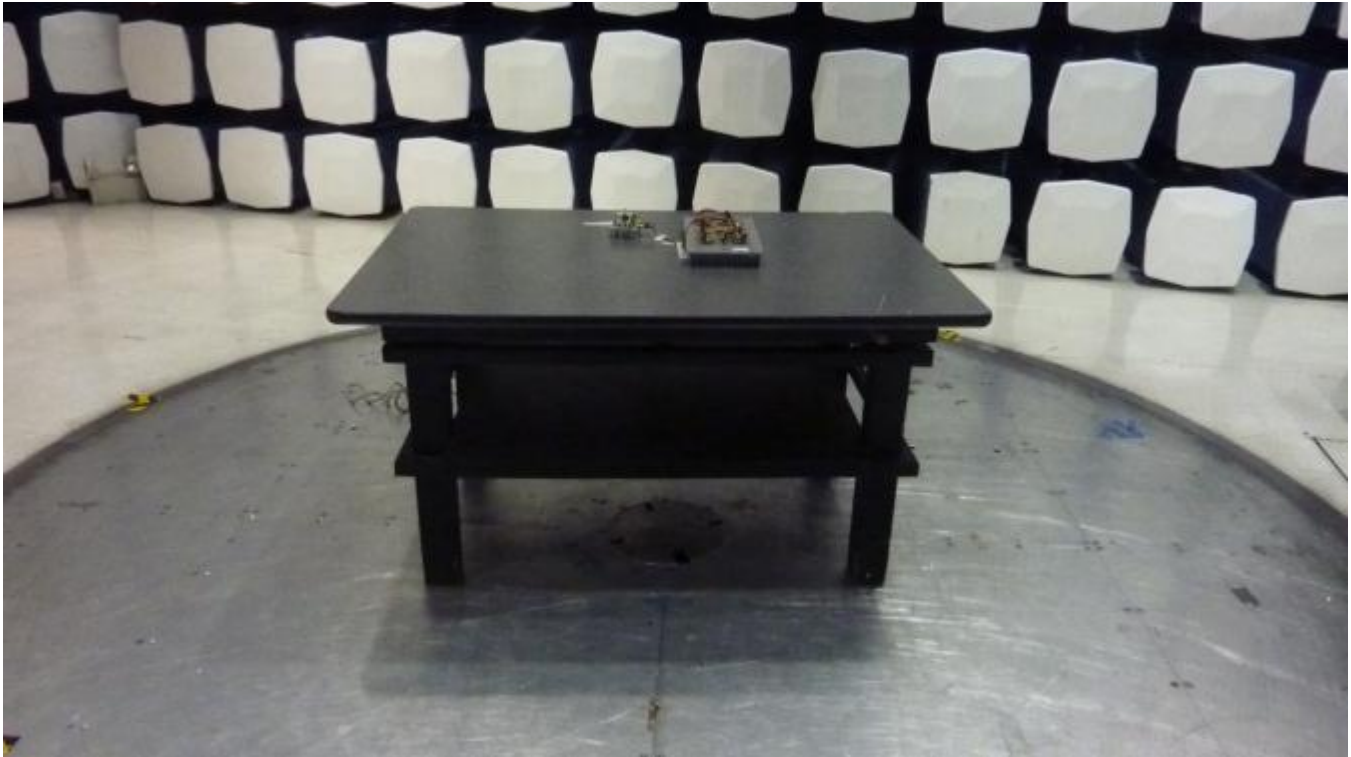
Figure 4 - Radiated Emissions Test Setup 30 - 1000 MHz - Front
