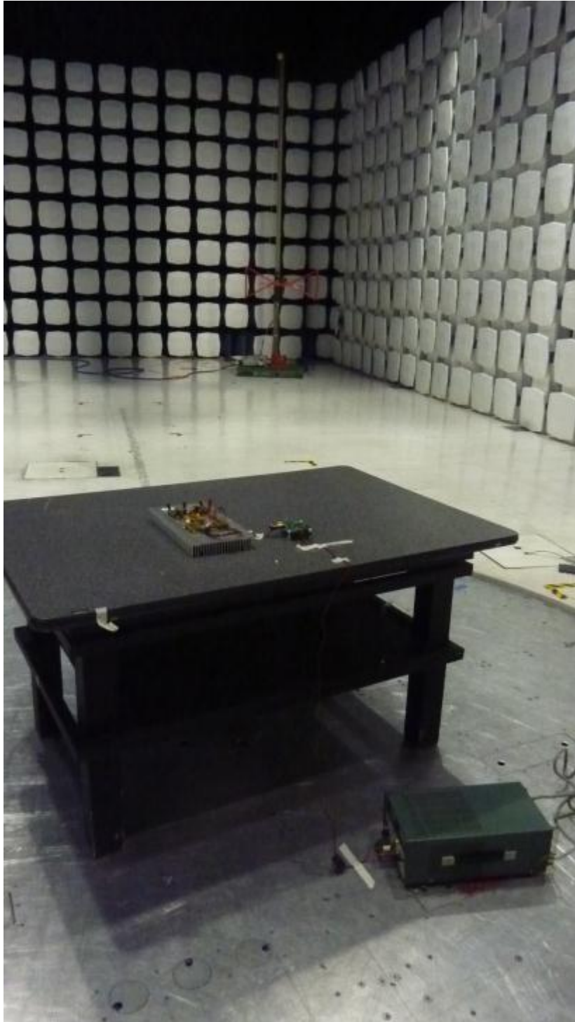
Figure 5 - Radiated Emissions Test Setup 30 - 1000 MHz - Back
