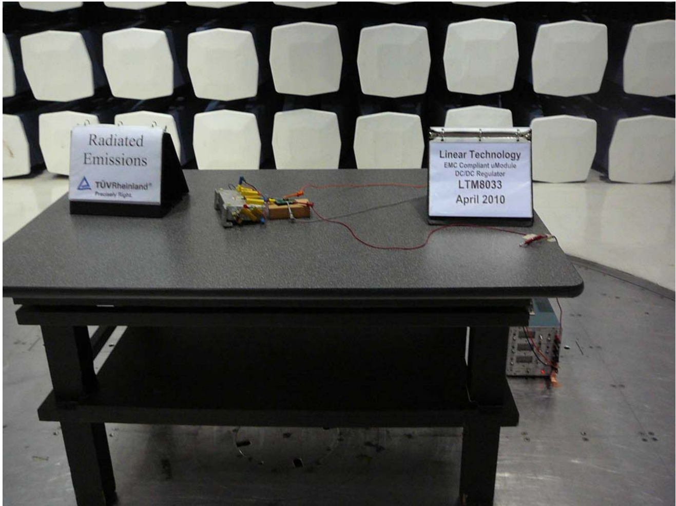
Figure 12 – Radiated Emissions CFG3 Test Setup – Front
