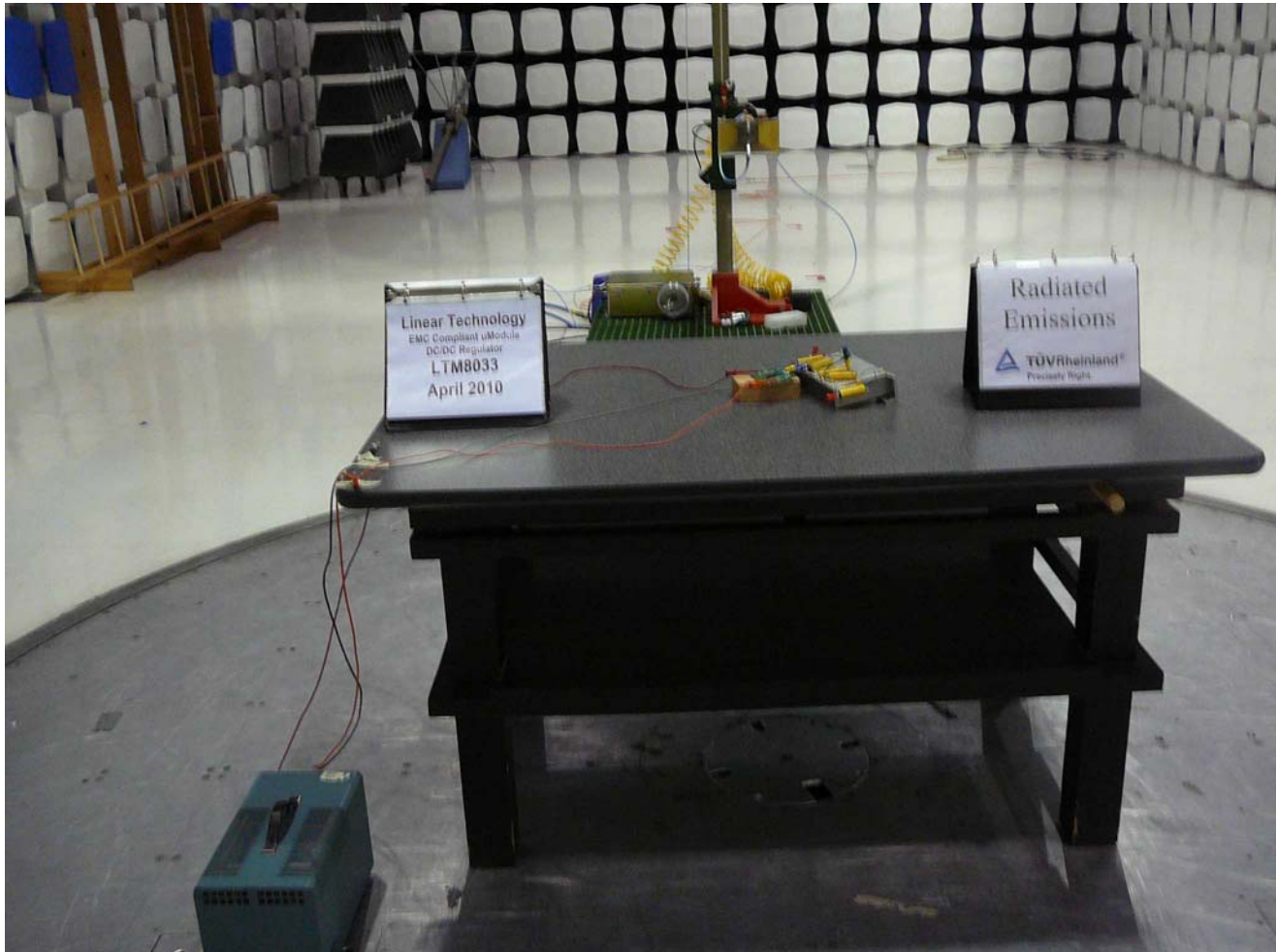
Figure 9 – Radiated Emissions 1000 - 6000 MHz CFG1 Test Setup – Back
