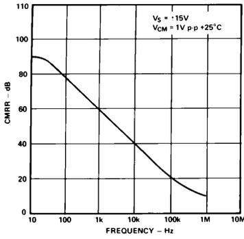
Figure 13. Common-Mode Rejection Ratio vs. Frequency
