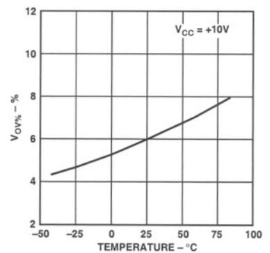
Figure 19. Overage Comparator Threshold ( $V_{OV\%}$ ) vs. Temperature
