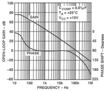
Figure 11. GM2 Open-Loop Gain and Phase vs. Frequency
