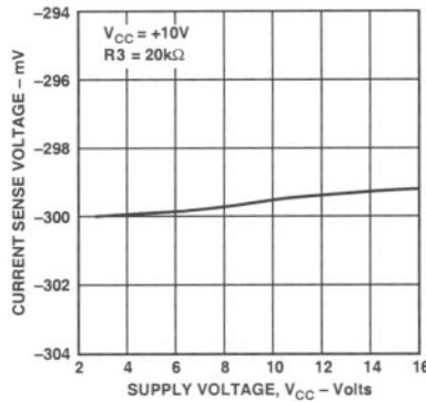
Figure 9. Full-Scale Current Sense Voltage vs.  $V_{CC}$
