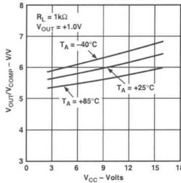
Figure 21. Output Gain ( $V_{OUT}/V_{COMP}$ ) vs.  $V_{CC}$
