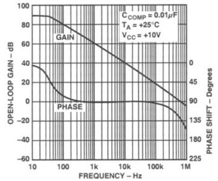
Figure 10. GM1 Open-Loop Gain and Phase vs. Frequency
