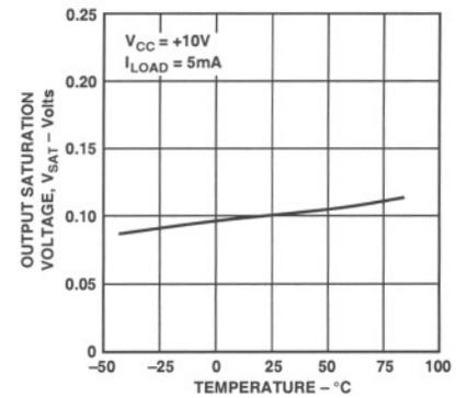
Figure 22.  $V_{SAT}$  vs. Temperature
