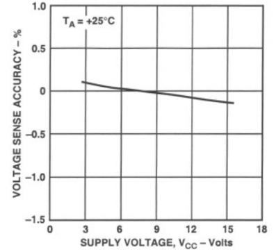
Figure 13. ADP3810 Voltage Sense Accuracy vs.  $V_{CC}$
