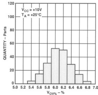
Figure 18. Overage Comparator Distribution ( $V_{OV\%}$ )
