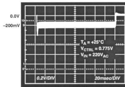
Figure 26. Charge Current Transient Response to Battery Connect/Disconnect
