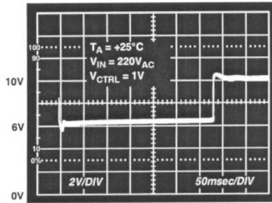
Figure 27. Output Voltage Transient Response to Battery Connect/Disconnect
