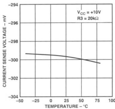
Figure 8. Full-Scale Current Sense Voltage vs. Temperature
