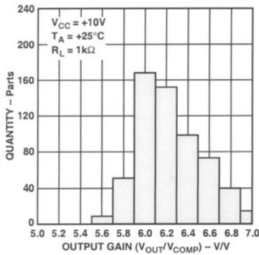
Figure 20. Output Gain ( $V_{OUT}/V_{COMP}$ ) Distribution
