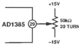
Figure 25b. AD1385 Offset Adjust Circuit
