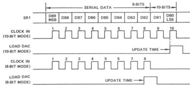
Figure 9. Timing Diagram for Serial 8- and 10-Bit Loading
