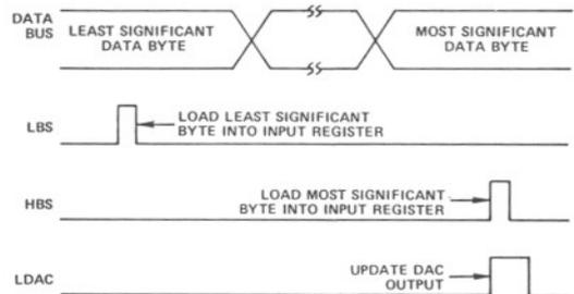
Figure 7. Timing Diagram
