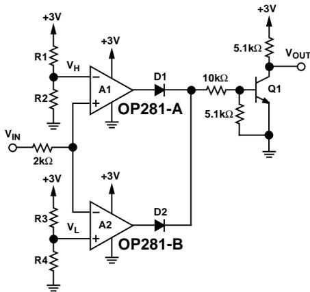
Figure 39. Using the OP281 as a Window Comparator
