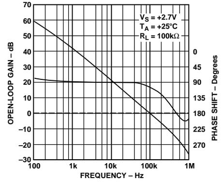
Figure 12. Open-Loop Gain and Phase vs. Frequency
