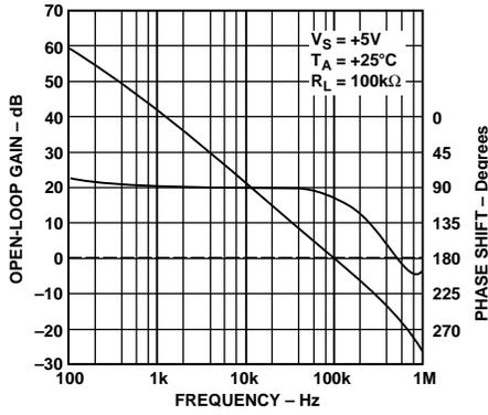
Figure 10. Open-Loop Gain and Phase vs. Frequency
