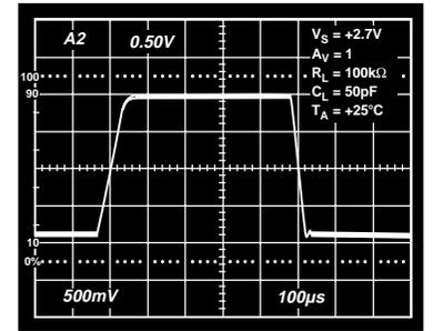
Figure 27. Large Signal Transient Response
