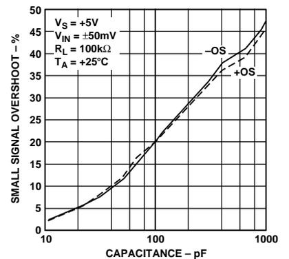
Figure 18. Small Signal Overshoot vs. Load Capacitance
