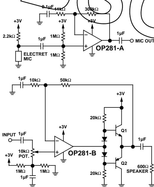
Figure 43. A Battery Powered Telephone Headset Two-Way Amplifier
