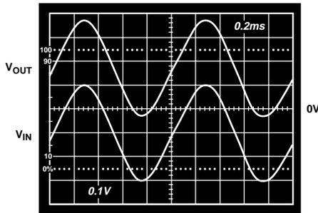
Figure 35. Input and Output Signals with  $V_{CM} < 0V$
