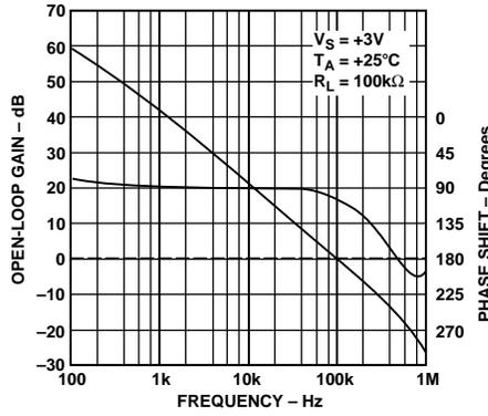
Figure 11. Open-Loop Gain and Phase vs. Frequency
