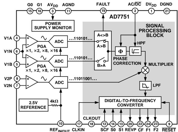
The AD7751 supplies average real power information on the low frequency outputs F1 and F2. These logic outputs may be used to directly drive an electromechanical counter or interface to an MCU. The CF logic output gives instantaneous real power information. This output is intended to be used for calibration purposes.
