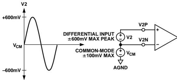
Figure 4. Maximum Signal Levels, Channel 2
