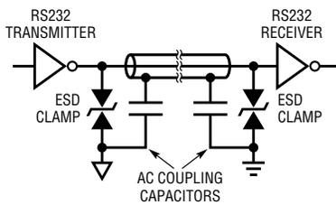
Figure 5. Older interface designs used external ESD clamps
