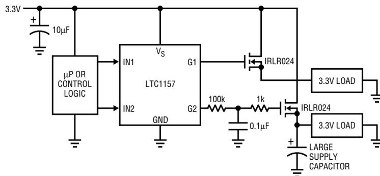
Figure 3. LTC1157 used to switch two 3.3V loads
