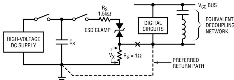
Figure 7. Circuit model for ESD current flow
