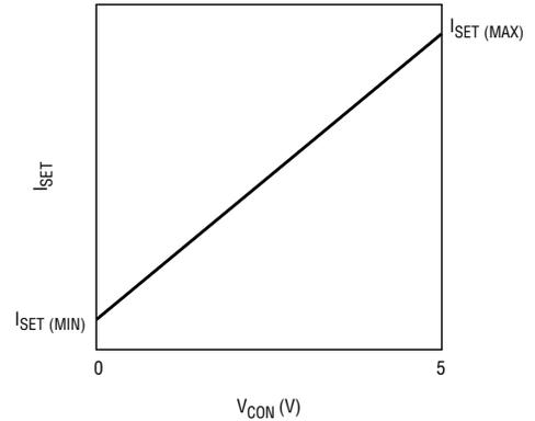
Figure 4. Voltage control of ISET with temperature compensation
