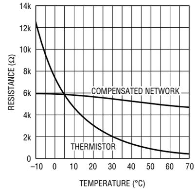
Figure 5. Thermistor and thermistor network resistance vs. temperature
