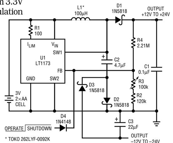
**Figure 1. DC to DC Converter Generates LCD Bias**
