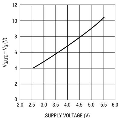
Figure 1. Gate voltage above supply vs. supply voltage
