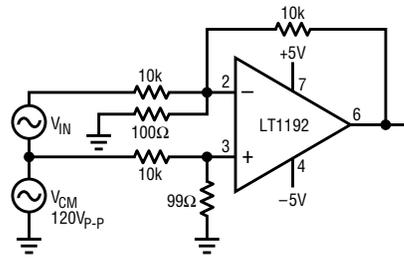
**Figure 10. 3.5MHz instrumentation amplifier rejects 120V<sub>p-p</sub>**
