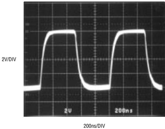
**Figure 11. Output of instrumentation amplifier with a 1MHz square wave riding on 120V<sub>p-p</sub> at the input**
