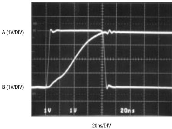
**Figure 9. Open-loop peak detector response**
