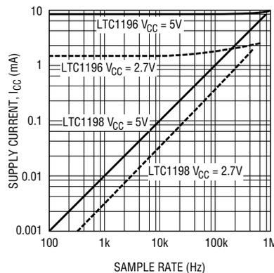
Figure 2. I<sub>CC</sub> vs. sample rate for LTC1196 and LTC1198 operating on 5V and 2.7V supplies
