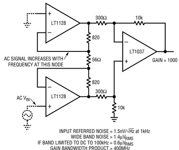
Figure 2. Three op amp, ultra-low noise instrumentation amplifier
