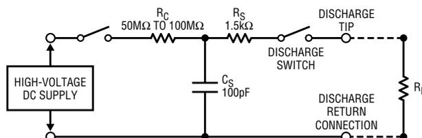
Figure 4. Human-body model circuit for ESD pulses
