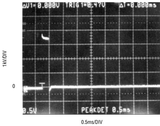
Figure 8. 10-mil spark gap limits ESD duration
