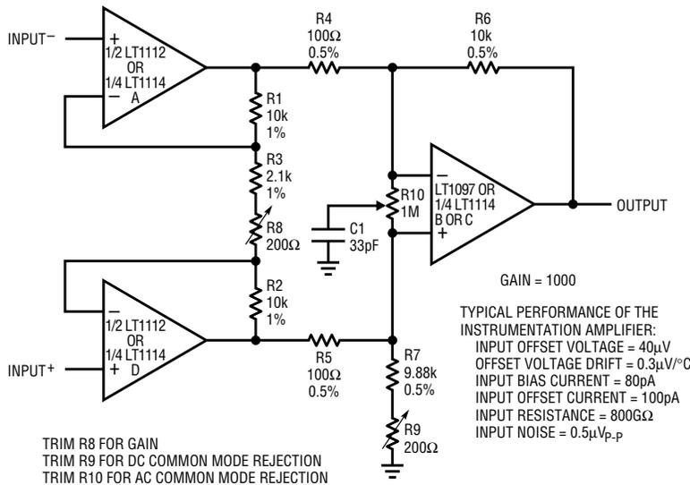
Figure 2. Three op amp instrumentation amp with gain = 100
